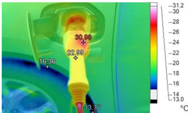
Fig. 4. Highest temperature of car charging socket during charging process.
