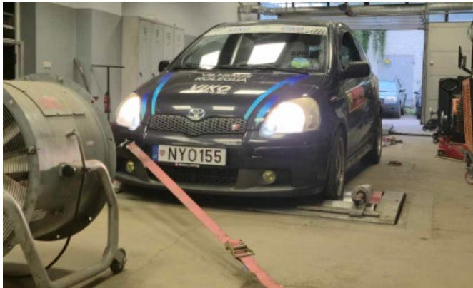
Fig. 4 Tested vehicle – TOYOTA YARIS T SPORT P1 strapped to a CARTEC LPS 2510 dyno for maximum power measurement.
